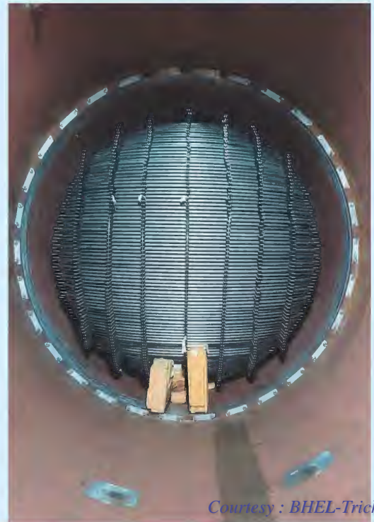
After complete insertion of all rows along with Anti-vibration U - tube supports and strips
